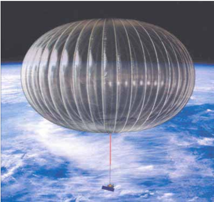
The super-pressure balloon, shown here as an artist's concept, is intended to operate for 60–100 days. Image credit: Columbia Scientific Balloon Facility
